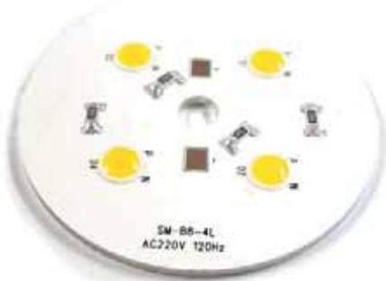
High voltage chip&COB Module
